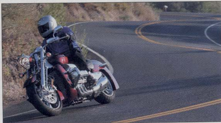
Left: Stock up on the chrome polish. Trailing bottom link front suspension is sturdy, supple and a styling TKO. Right: Cornering clearance is similar to VTX's.
