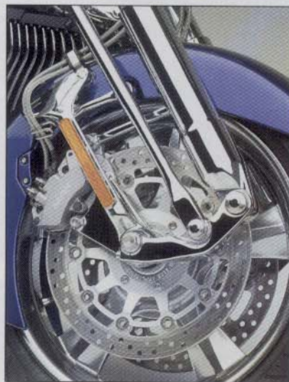
Top and above: Rune's trailing bottom-link front suspension transfers loads through pushrods and linkage to two upper shocks—one housing the main spring and one a sub-spring and damping system. Linked, triple disc brakes are the largest ever fitted on a production Honda. Remote steering lock is actuated by a lever with key in off position; it unlocks automatically when ignition is turned on.
