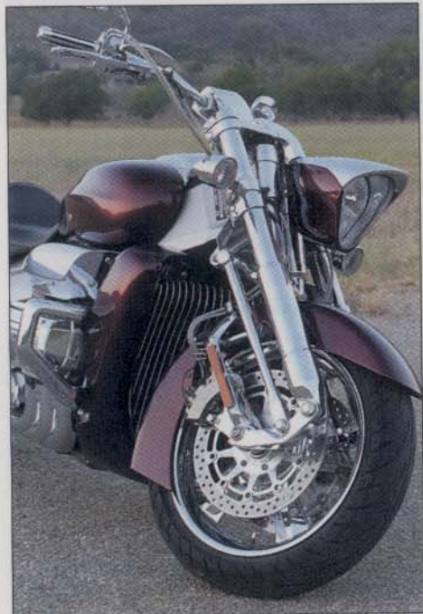
Left: Stock up on the chrome polish. Trailing bottom link front suspension is sturdy, supple and a styling TKO. Right: Cornering clearance is similar to VTX's.
