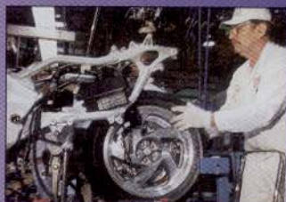
Fewer robots and a more flexible assembly line accommodate limited-production machines like the Rune quite well.
