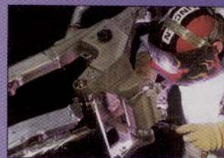
Some of the complex welds on the Wing's aluminum frame are done by skilled hands rather than robots.
